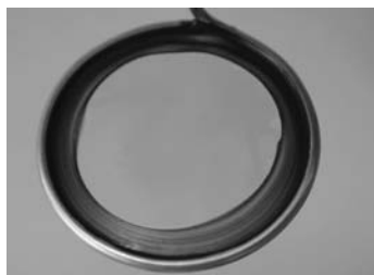
Figure 2. Photograph of a PVA thin film containing MWCNT prepared in the magnetically simulated microgravity ( 5\text{ T} , -900\text{ T}^2\text{ m}^{-1} ). The central area looks like a hole because of too thin thickness, but the clear layer with carbon nanotubes has been prepared.
